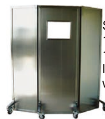
Steel mobile barrier 1800x900x900mm 1mmpb or 2mmpb lead glass viewing window 200x300mm
